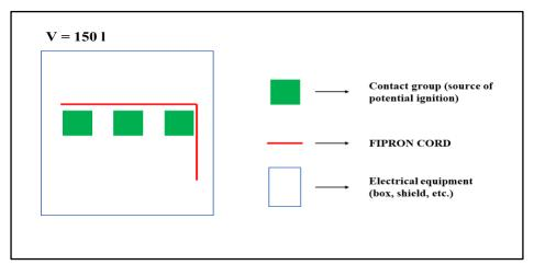
Legend: contact group; FIPRON CORD; Electrical equipment (switchboard, fuse box, etc.)
