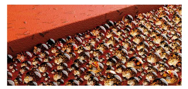
When the capsules reach the initiation temperature, they burst and release the active agent. Active agents can extinguish class A, B and E fires. Until the initiation temperature is reached, the microcapsules remain intact in the ambient temperature range of -50 °C to +80 °C.
